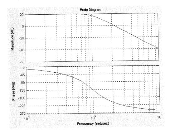
a) What are the gain and phase margins of this system? Will it be stable when connected in the above feedback system with K(s) = 1?
