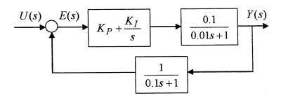
a) Determine the range of gains  $K_I$  and  $K_P$  that will lead to a stable closed-loop system.
