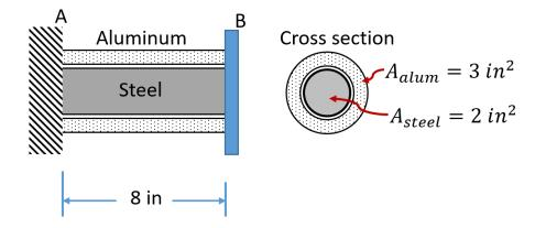
b) Find the internal stress in the steel bar when the temperature reaches 145°F.
