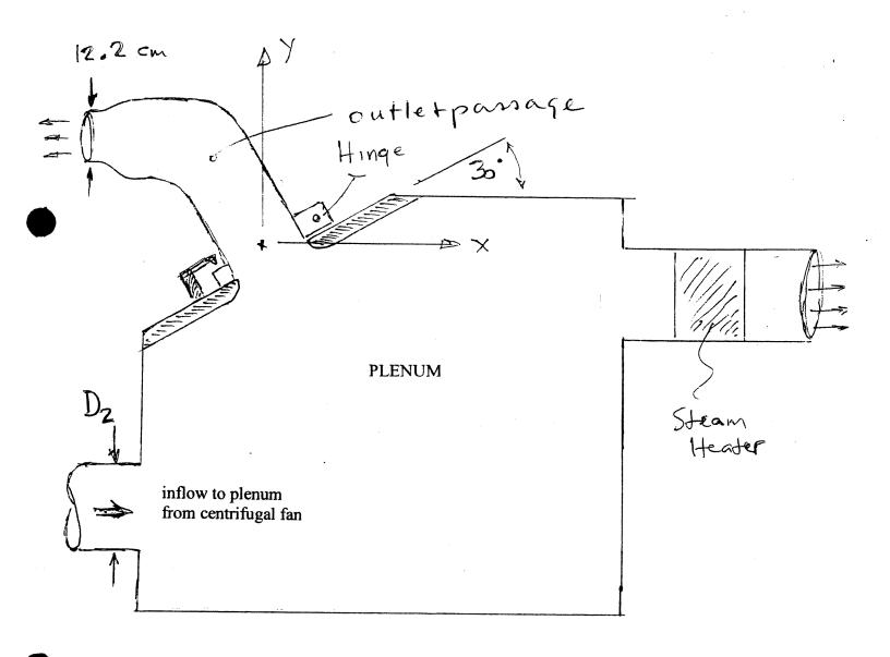
(20) c) Eighty percent of the flow into the plenum exhausts through the "outlet passage" shown on the preceding sketch.
